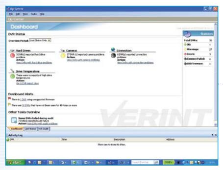
The Op-Center dashboard displays DVR information in an easy-to-read, color-coded format, with red, yellow, and green indicators, so users can see at a glance the operational status of all networked DVRs.
